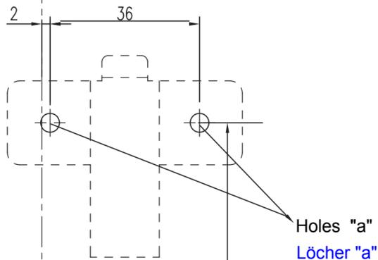
1. Check if your cabinet has a smooth, flat bottom and right size, and tape the template onto the bottom plane of cabinet.
