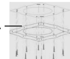
2. Drill the holes marked on the wall and insert the plugs for fixing the mounting plate.
