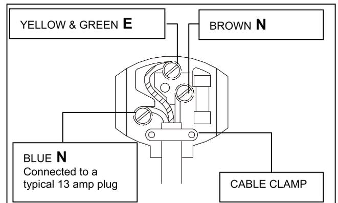
1. The YELLOW & GREEN wire must be connected to the terminal in the plug which is marked with the letter **E**
